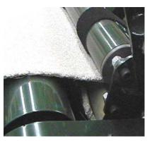
$\blacktriangleright$  While gently holding this Handle in place, press the Jog Button to continue the advancement of the carpet. You will only have to hold the Handle in place for 1 or 2 seconds at which time you will see the plates actually force the carpet around the core. Once you see the carpet is starting to wrap around the core, release the Handle to its original position.
