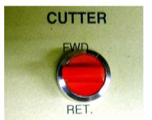
$\succ$  Because it is a Two-Way Cutter, you do not have to return the Cutting Bar back to the home end of the machine for the next cut.
