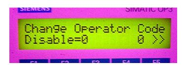
Feature: This screen allows you to enter a pass code for safety and security reasons. The machine will not be operable unless this Operator Code is keyed in. **DO NOT** FORGET YOUR PASS CODE IF YOU CHOOSE TO USE ONE!
