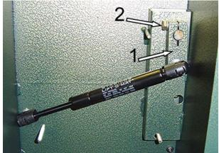
This photo shows the position the Counter Weight Bracket (#1) should be in with the Counter Weight Wheel in the **DOWN** position. To make your adjustment loosen the Bolt (#2) and put your Counter Weight Wheel Down so the Bracket is in this vertical position.
