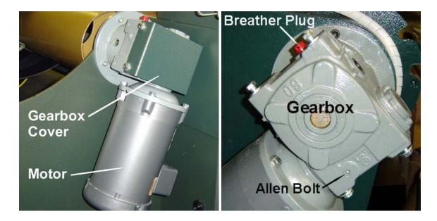
**IMPORTANT NOTE:** The Counter on your machine is programmed to remind you to change the oil after the machine has been used for a set amount of hours. The oil must be changed when this message comes up or once a year - whichever comes first.
